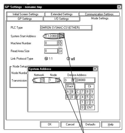
The System Start Address is allocated to the PLC node entered here. Set the Network Address and Node Address to the same address values as set in the Destination Node Infomation. (Set in the [MODE SETTINGS] -> [NETWORK SETTINGS].).
